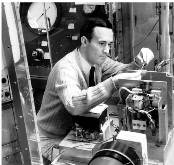
Figure 6. Luigi T. DeLuca in Summerfield's laboratory adjusting his CO 2 laser apparatus for energetic-material ignition experiments. 1971.
